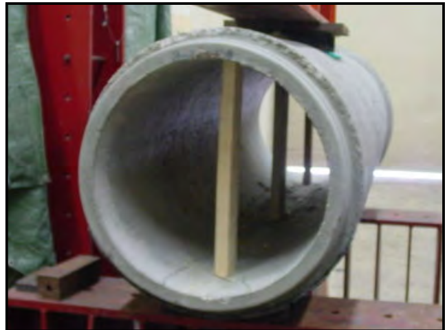
Figure 6. Test 3 of Specimen 3, with all but four vertical stiffeners removed.
