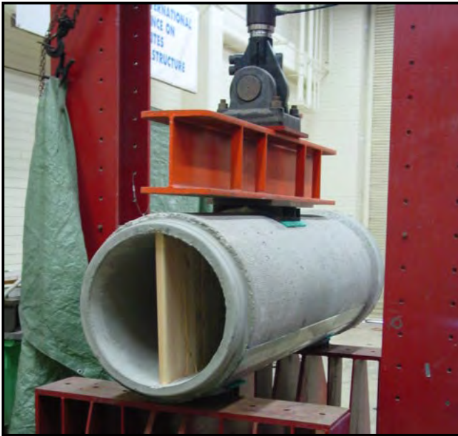
Figure 3. Wood stiffeners used for specimen 3.
