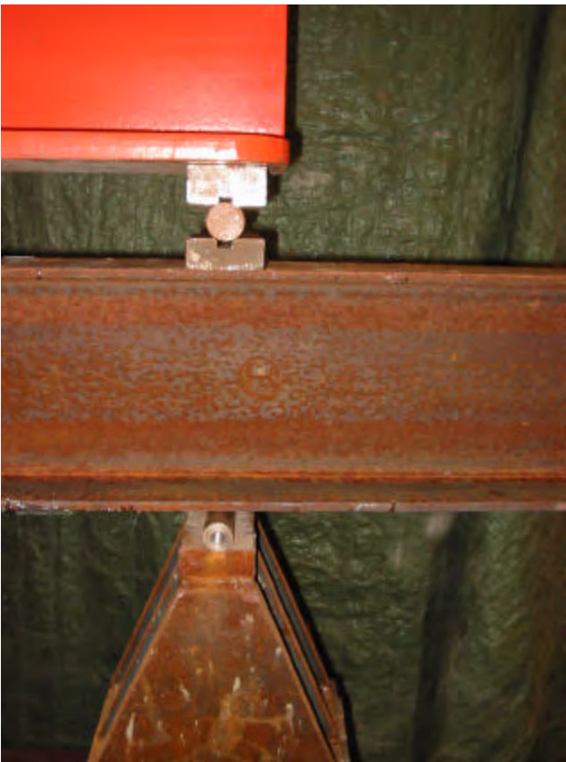
Figure 4. Rollers used during testing. Top roller is not shown in actual location used for testing.
