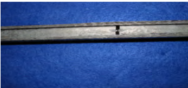
Figure 7. Post-test close-up of the cut made in the steel plate.
