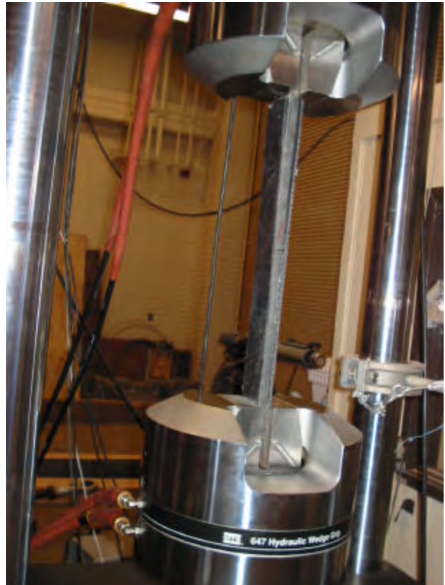
Figure 10. Specimen shown in MTS testing machine with gripping pressure applied.
